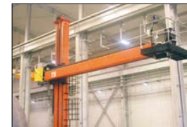
All Time 6m x 7m HEAVY DUTY Manipulator built with walkway on boom and safety ladder
