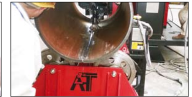
Internal SAW head for part inside diameter as little as 400mm
