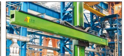
Modified All Time 7m x 7m HEAVY DUTY Manipulator with precise on boom carriage and deep groove SAW head
