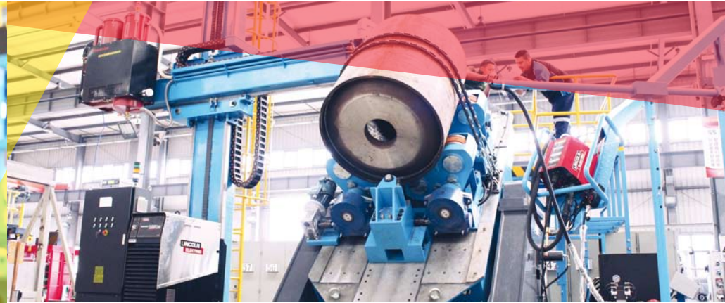
OD/ID Fillet Welder for heavy pulleys
