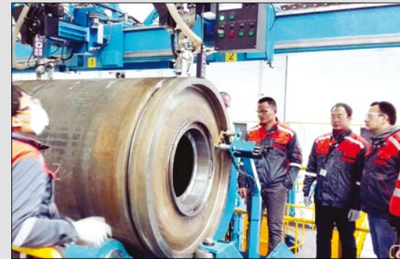
OD butt + ID fillet welder for heavy pulleys
