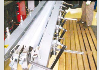
Aluminum beam clamped on jig prior welding
