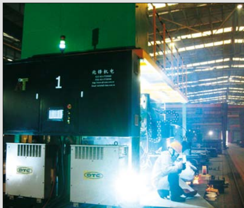
2 power supplies for independent weld head assemblies on each side (front & back) with a central control with touch screen control
