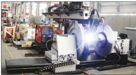
All Time CTP PRECISION Manipulator to provide precise positioning of welding arc for TIG or PAW applications
