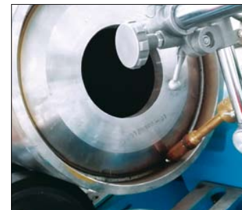
Outside Fillet Welder for light pulleys
