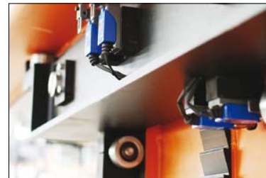
Limit switches and anti-fall mechanism for safety
