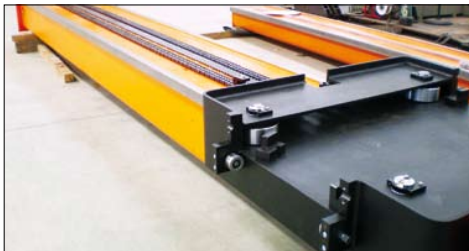
Wear resistant chrome molly guide way specially welded on column and boom for long time accurate performance with minimum maintenance
