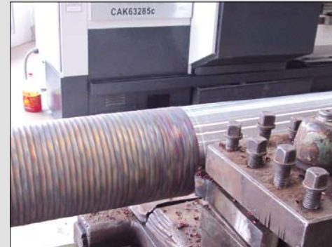
Roll Surfacing by SAW
