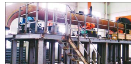
ID/DD Pipe Welder for large diameter heavy pipes
