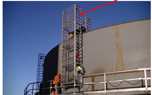
Manual chain drive on both sides allows a single operator to move the unit into place. The drive wheels swivel to allow for easier travel on various tank diameters.
