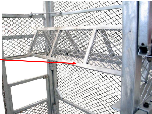
Additional cross members have been added from the top to the bottom of the frame and spaced to work as Ladder Rungs built into the Shell buggy frame so the operator can easily and safely climb between the levels.
